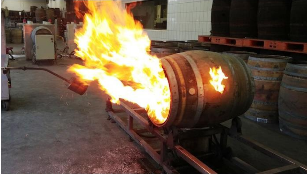
A Kavalan whisky barrel being recharred. (image via Jake Emen)
