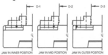
Minimum gripping diameter using long bite of jaw with master jaw in minimum effective gripping position.
