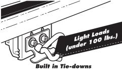
Clamp tie-downs for light to moderate loads (100 lbs max.) can be used whether tonno is in place or not.
