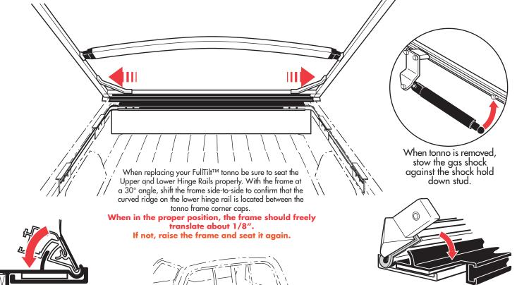
Make sure that Upper Hinge Rail Assembly slides easily over ridge on Lower Hinge Rail.
