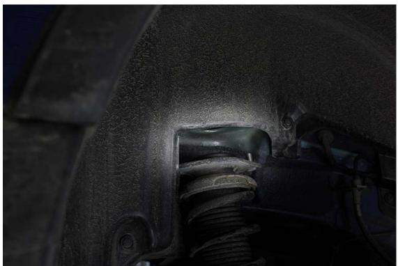
Note: You can use a bolt to remove paint deposits that might be in the bolt threads. (Tap M10x1.25)
