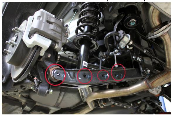
Note: You must remove the carpet and plastic covers in the trunk to have access to the suspension bolts.
