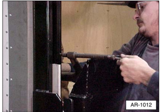
Illustration 4. Clamp the liftgate to the truck body side rails.
