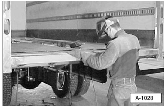
Illustration 2. Find and mark the center of truck's rear sill.
