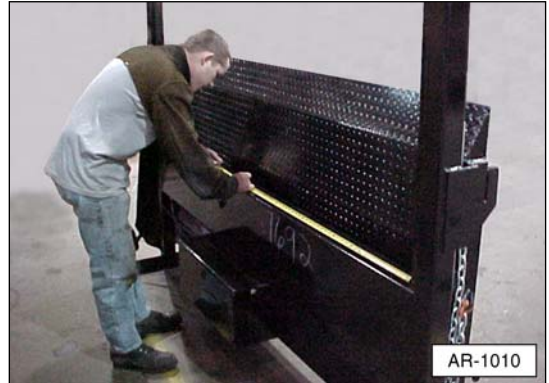
Illustration 1. Mark the centerline of liftgate.
