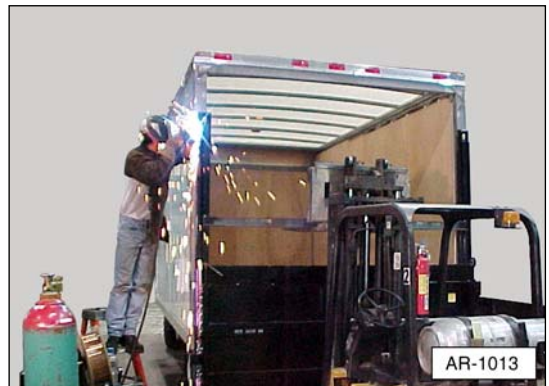
Illustration 5a. Tack weld the H-frame columns and the housing to the rear sill.
