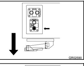
Push Open Switch to move Platform to working position.
