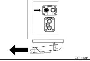
Lower Platform to ground. Open Platform Extension and Loading Ramps manually. Note! Use handle to open Platform Extension.
