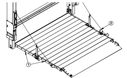
If liftgate is WDVBG, check additional bolts, fasteners and pins are tight and secure:
