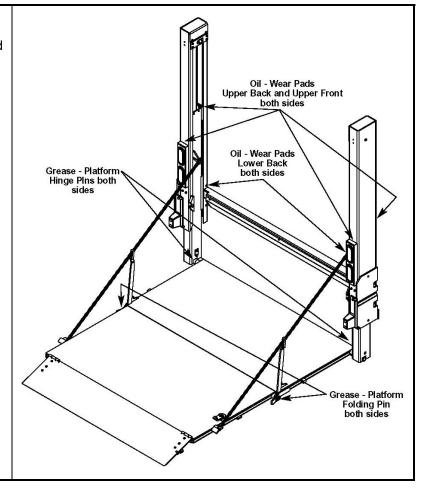
If the liftgate is a WDVBG, the additional points on the liftgate that require lubrication are the points indicated in the graphic to the right. These should be lubricated approximately once every three (3) months.
