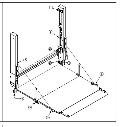
If liftgate has Aluminum Platform, check additional bolts, fasteners and pins are tight and secure:
