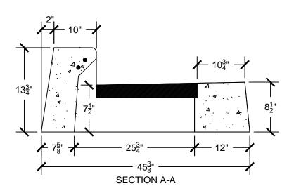
CLASS "FSC" SELF-CONSOLIDATING CONCRETE 4,000 PSI
