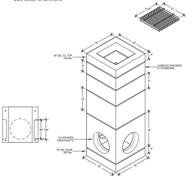
CLASS "FSC" SELF-CONSOLIDATING CONCRETE 4,000 PSI
