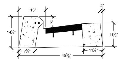
CLASS "FSC" SELF-CONSOLIDATING CONCRETE 4,000 PSI
