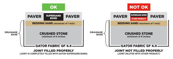
NEVER USE SUPERSAND BOND WHEN PAVERS ARE INSTALLED ON A CONCRETE SLAB –
