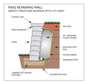
\*Important! Walls 4' and higher; terraced walls, sites with weak or wet soils, slopes and other loading conditions require special considerations and construction techniques, including the use of geogrid. We recommend you consult a qualified soils engineer for these situations.
