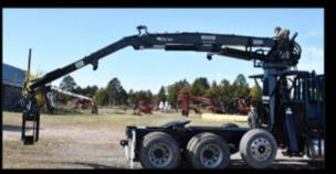
The Hood S-8000 Series high-pressure knuckle boom loader provides an efficient one-man solution to material-handling challenges. Move pole-length trees or utility poles -- or any job calling for extra lift power or multiple heeling accommodations.
