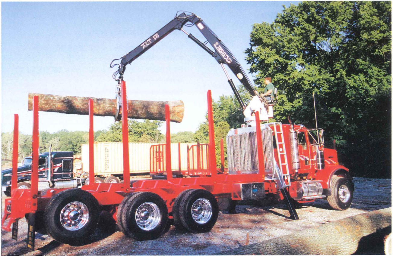
The Model XLT 80 Loader with 6,900 Lbs. Net Weight. 23' Boom with 4' Extension
