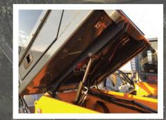
PUSH BUTTON CAB TILT FOR EASY ACCESS TO COMPONENTS & HYDRAULIC OIL FILLING PUMP
