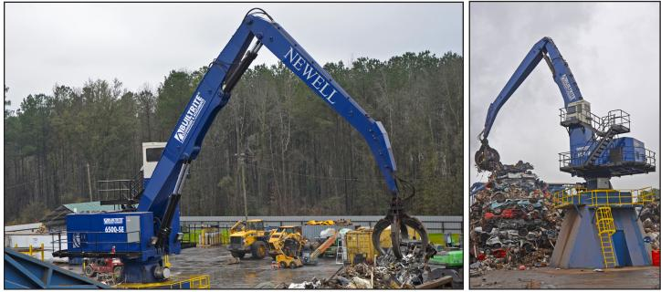
6500-SE With Two-Piece Boom, Full Catwalk/Stairway (note: Pedestal foundation base (blue with yellow ladder) is <u>not</u> included with the machine.)
